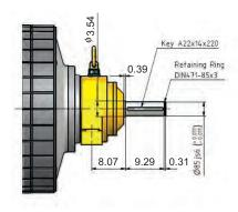
\* All dimensions are in imperial units, except for brake shaft diameter, key, and retaining ring, which are metric.
